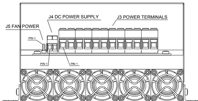
*J5 FAN POWER CONNECTOR* is the power connector for the fan system. This connector sinks directly the power from J4 connector. (Not used on natural cooling versions)
